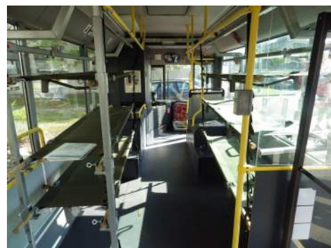
■ Above, seats are removed from a bus, and the three level stretcher bunks installed. Below, the kit as stand alone
