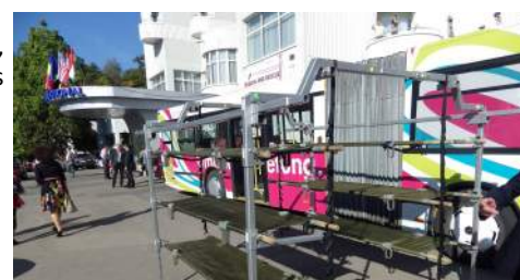
■ Above, seats are removed from a bus, and the three level stretcher bunks installed. Below, the kit as stand alone
